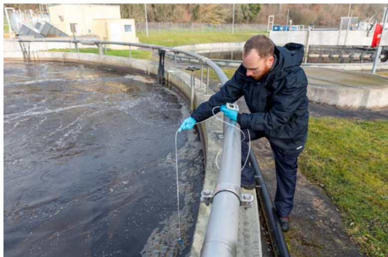
Fig. 4 Occasional measurement at process points where no on-line measurement is installed
