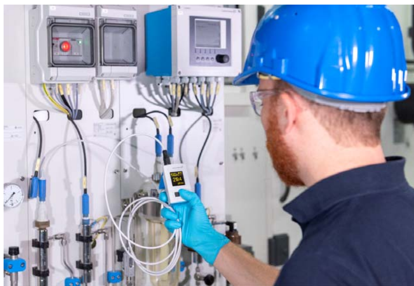
Fig. 2 Robust grab sample measurement directly at the sampling point
